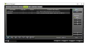
6.7 Click the tab of "DMX devices", set port status to "ON" if connected successfully. Now, you can use computer to control lamps via ArtNet-DMX-1.
