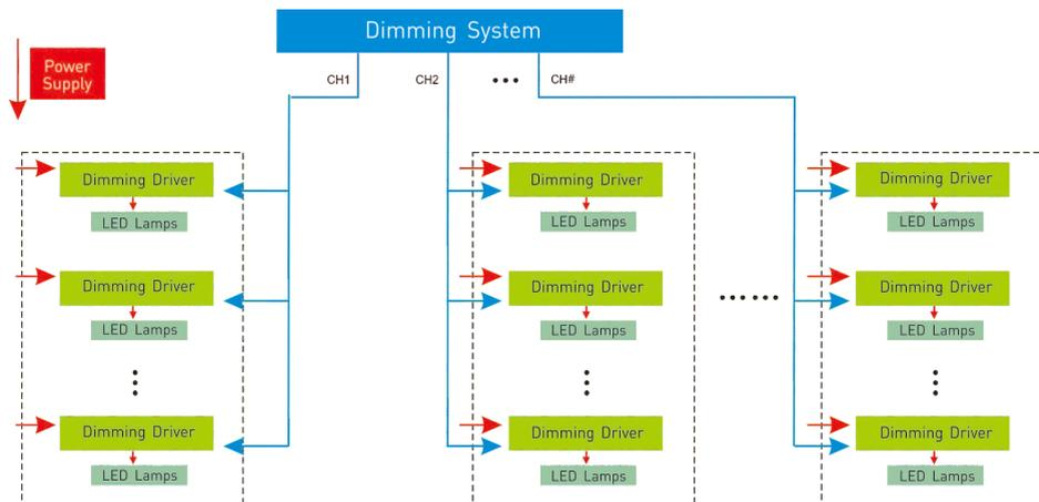
The default design doesn't support the 1-10V and push dimming that work together, if you want them to work together, please mark down when placing a order.
