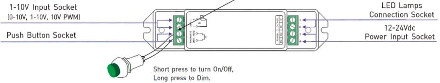
12V lamp connected, loads 0~72W(12V).
