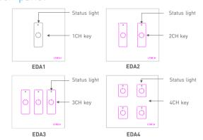
\* Short press: switch; long press: dimming (suitable for unicast, broadcast and group mode).
