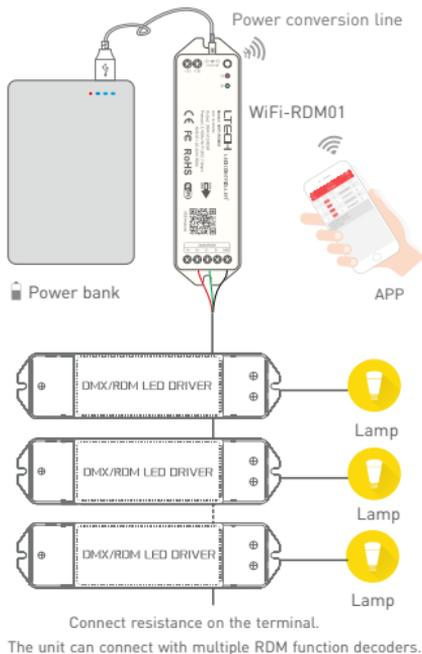
★ The product can be powered by power bank or 5-24V adapter through power conversion line.
