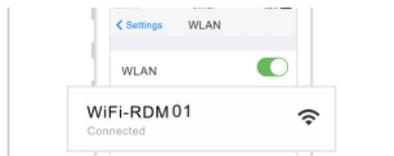
Attn: if the phone failed to search "WiFi-RDM01" SSID, please reboot the power supply, and reconnect WiFi when the communication light is off.
