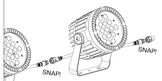
For waterproof connection make sure that the last fixture has the endcap connector fixed to the output connector
