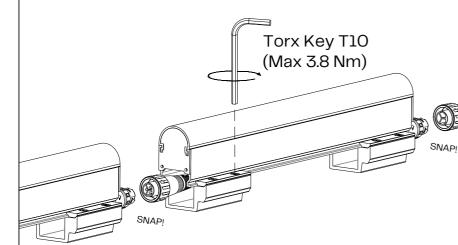
For waterproof connection make sure that the last fixture has the endcap connector fixed to the last output connector
