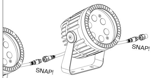
For waterproof connection make sure that the last fixture has the endcap connector fixed to the output connector
