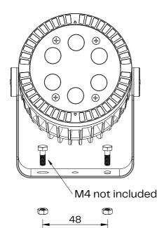
Use a Hex key to fully secure the fixture when the desired angle has been set.
