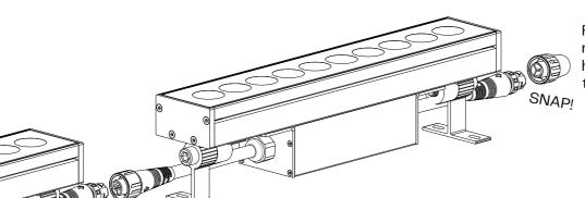
For waterproof connection make sure that the last fixture has the endcap connector fixed to the output connector
