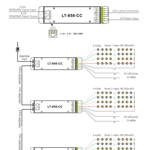
\* If the recoil effect occurs because of longer signal line or bad line quality, please try to connect 0.25W 90-120Ω terminal resistor at the end of each line.
