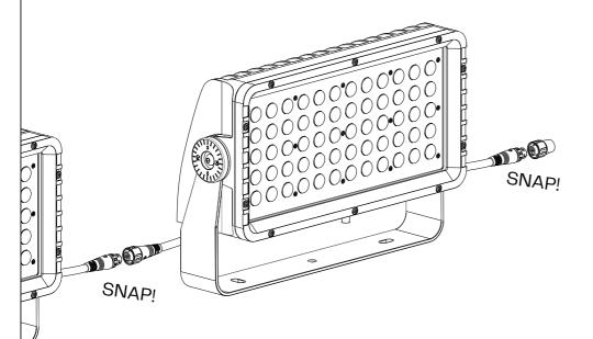
For waterproof connection make sure that the last fixture has the endcap connector fixed to the output connector
