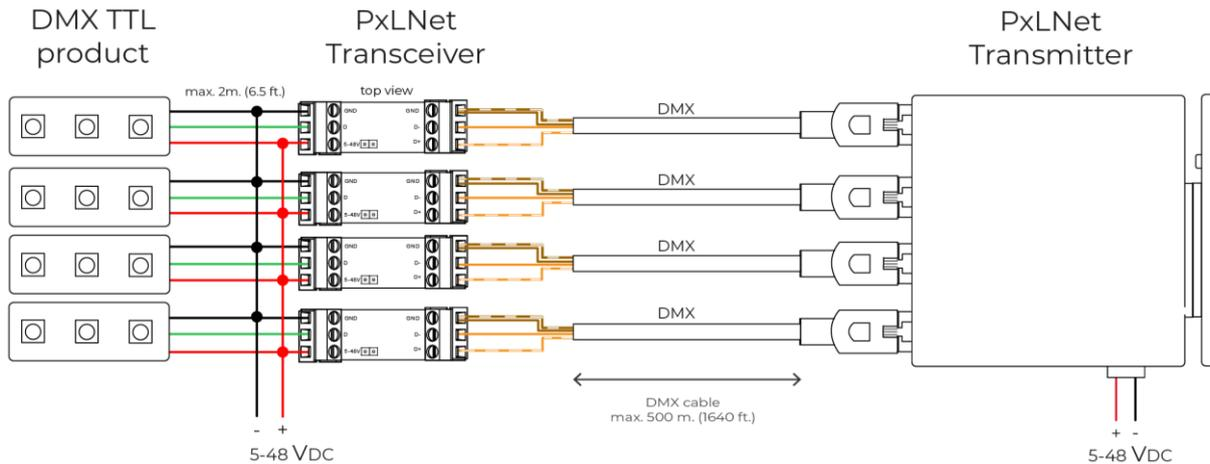
Using an external DMX signal, connected to a PxLNet Transceiver which is connected to a DMX TTL controlled LED product. The DMX signal can be soldered, as indicated in the drawing or can be inserted in the RJ45 bus on the top side (DMX pinout according to USITT standard, see page 5)
