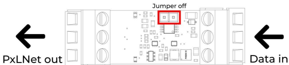
Connect a network cable to the RJ45 bus and connect it to the next PxLNet Transceiver in receiving mode (Rx).
