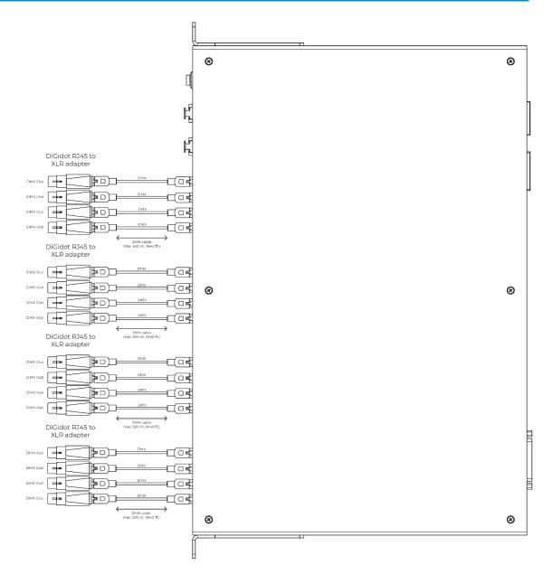
Max. 512 channels per combined DMX port | DMX cable max 500 m. (1640 ft.)
