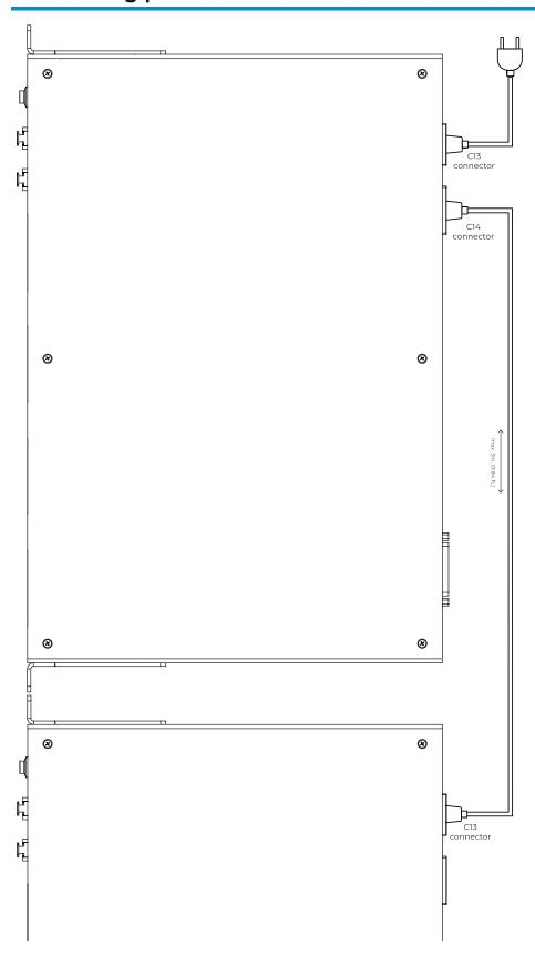
Connect the DiGidot PxLNet Node to a power source and switch the device on with the power switch on the front. You can also daisy chain the power cable with a C14 male to C13 female cable.
