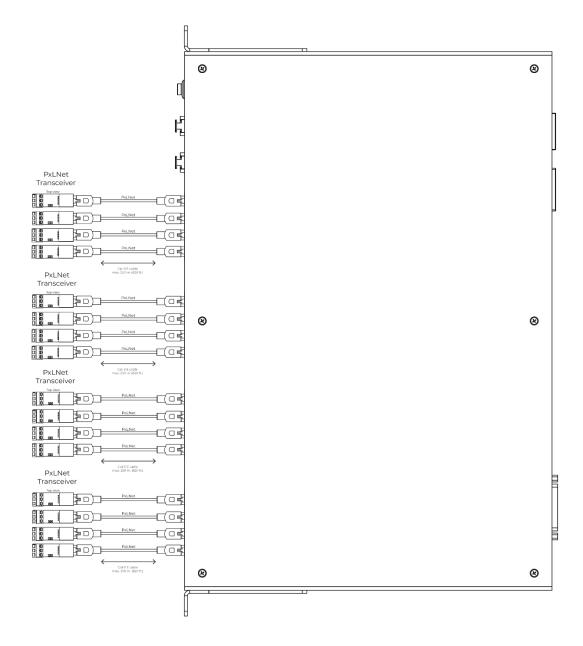
Average recommendation is max. 3 SPI universes per port (check the SPI Performance guide for max. load per IC)
