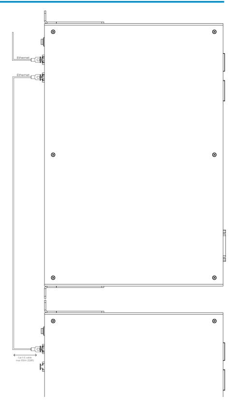
The DiGidot PxLNet Node has a built-in Gigabit ethernet switch that allows multiple units to be daisy chained. It's recommended to not daisy chain more than 8 PxLNet Nodes.
