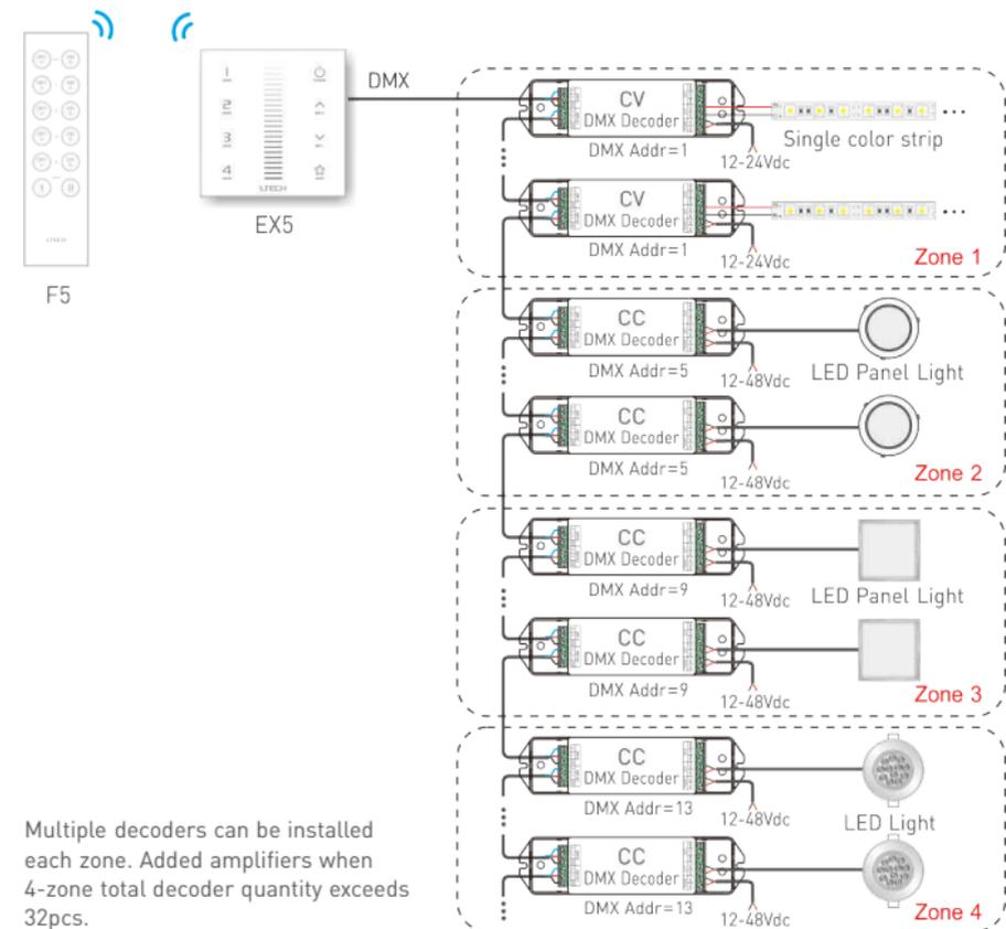
Multiple decoders can be installed each zone. Added amplifiers when 4-zone total decoder quantity exceeds 32pcs.
