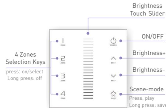
\* When the touch panel is off, Long press to turn on/off the buzzer
