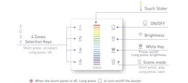
When the touch panel is on ,Long press  $\overset{\text{\tiny{(1)}}}{\bigcirc}$  to match code.
