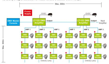
4.3 Example: Connection for signal amplifier in long distance:
