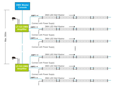
4.2. Example: Signal distribution for master console & decoder & DMX lamps:
