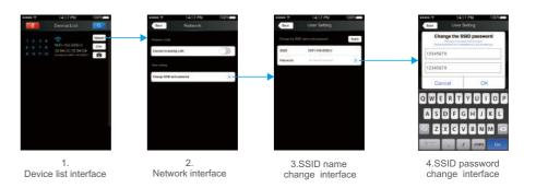
Attn]: Direct connection of using wifi-104 as a router, exit the App after the SSID name and the password changed, reconnect the WiFi-104 on the mobile devices.
