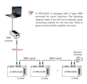
\* If the recoil effect occurs because of longer signal line or bad line quality, please try to connect 0.25W 90-120 $\Omega$  terminal resistor at the end of each line.
