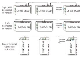
These 3 terminals can be connected in a mixed way.
