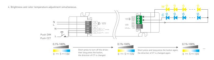
\* Dimming interface priority: First 0-10V, next Push DIM/CCT.
