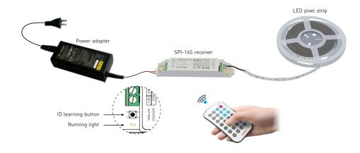
LED pixel strip wiring diagram:
