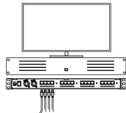
With the use of the DiGidot PxLNet Node up to 250mtr cable length for data to the PxLNet Transceiver (PT) can be achieved
