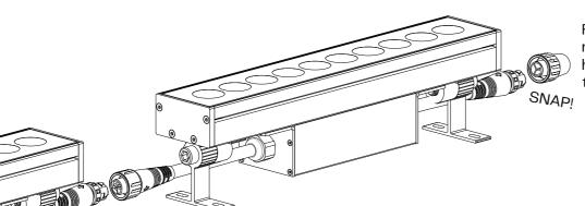
For waterproof connection make sure that the last fixture has the endcap connector fixed to the output connector
