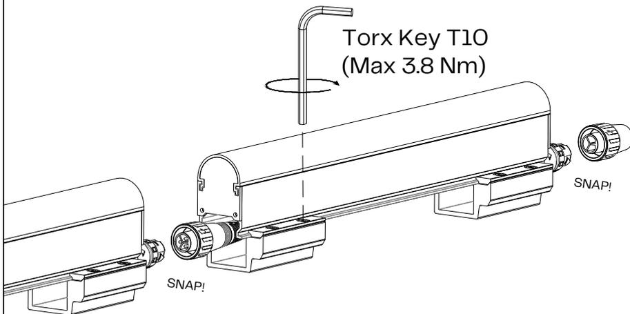
For waterproof connection make sure that the last fixture has the endcap connector fixed to the last output connector
