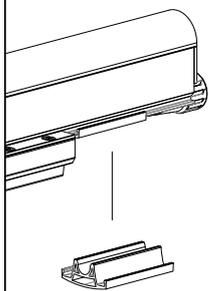
When the fixture is installed cables are connected between the fixtures the cable guide be placed to make sure the cable will not make any unnecessary movement
