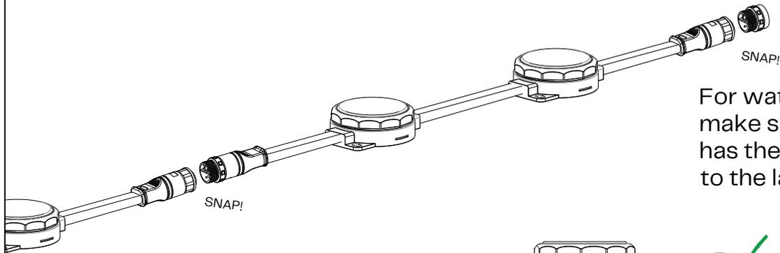
For waterproof connection make sure that the last fixture has the endcap connector fixed to the last output connector
