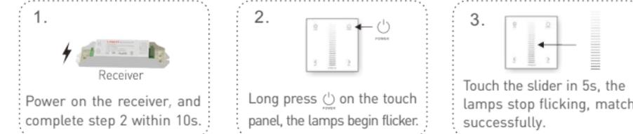
Method 2 : When the touch panel is on and the wiring between the receiver and the lamps are correctly,
