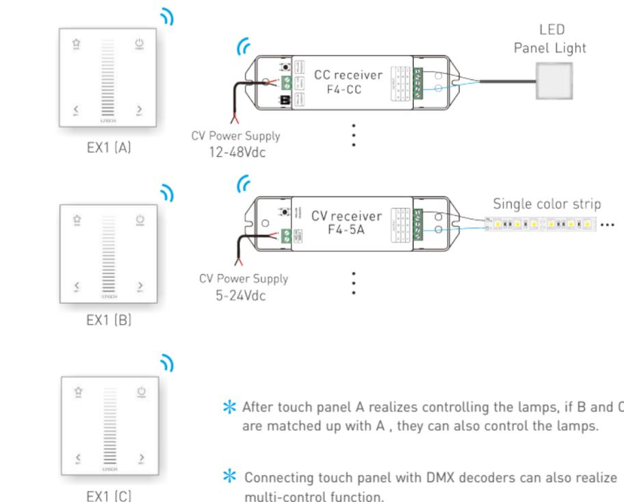
\* After touch panel A realizes controlling the lamps, if B and C are matched up with A, they can also control the lamps.
