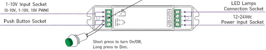
12V lamp connected, loads 0~72W(12V).
