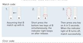
Press the bottom two keys of B simultaneously (about 6 seconds) until the indicator light keeps on, deactivated matching successfully.
