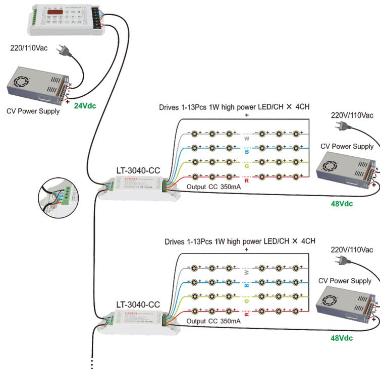
3.2 Repeaters connected to DMX constant current decoder:
