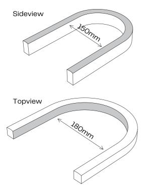
When using mounting profiles make sure the neonflex is pushed in from one side.
